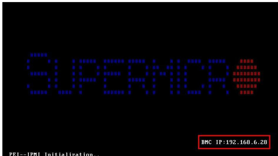
Fig – Finding IPMI/BMC IP
