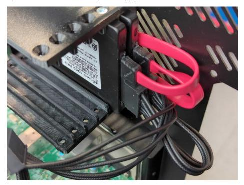
As mentioned previously, the purpose of the two end-pieces is to hold the SSD screws in place during shipping. They can be discarded and any unused SSD screws can be kept aside for future SSDs.
