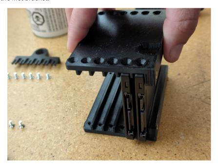
8. Secure the second bracket to the other side of the SSDs with the smaller screws.
