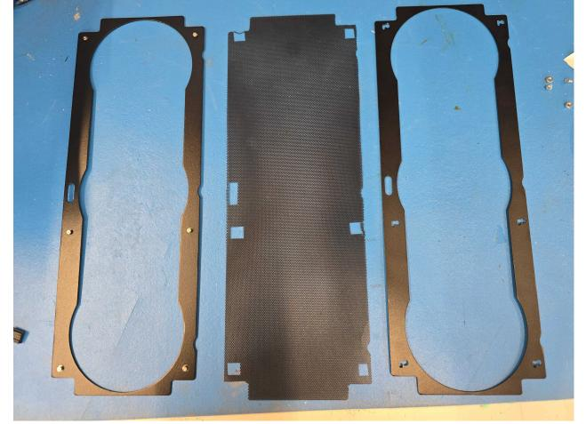
• Take the middle piece(filter) and lay it on top of the left most piece lining up the holes, then layer the right piece on top and lock it into place by sliding it to the right then up. It
