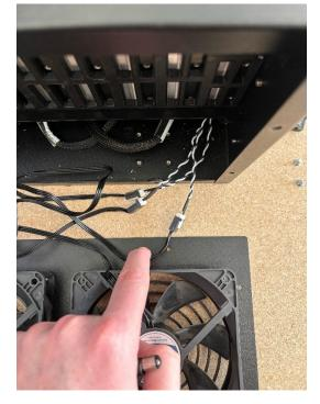
9. Turn the front plat over and remove the 12 screws to remove the fans.
