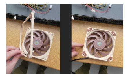
6. Mount 3 fans to the front plate with the vibration plates attached to the fans using screws from step two, with the wires coming from the bottom of all (3) fans. (Be sure rubber grommets stay between fans and front plate and do not over tighten)
