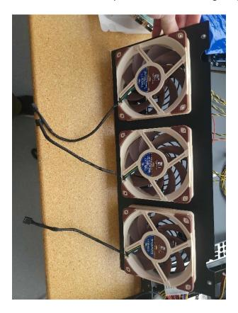
7. Connect the cables of each of the 3 front fans to any of the 8 slots on the fan hub. This will later provide the fans with power.
