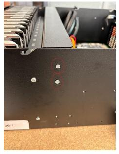
3. Slide the center bracket upwards and remove it from the chassis.
