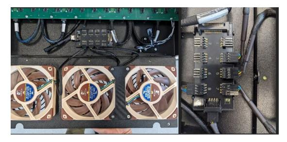
8. Apply double-sided tape to the back of the fan controller and place on the left side of the chassis next to the motherboard. [This can be removed while connecting cables.]
