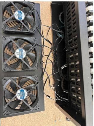
8. Locate and disconnect the cables from the front plate fans.
