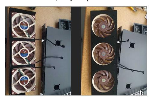
4. Connect the 3 rear fan cables to the 3-way splitter cable provided.
