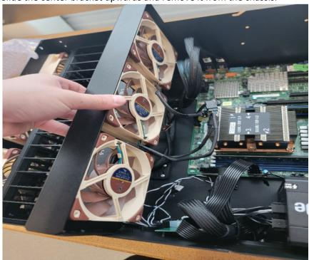
4. Remove the 12 screws securing the fans to the bracket.
