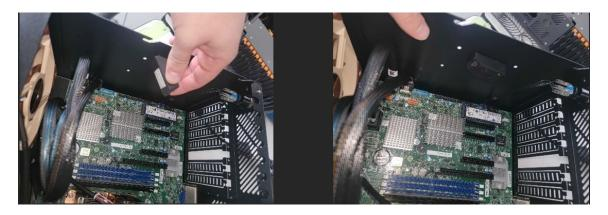
9. Take an extension cable and plug that into the power port on the fan hub. Feed the other end under the components leading to the motherboard and plug into another extension cable that you will connect to the fan controller.
