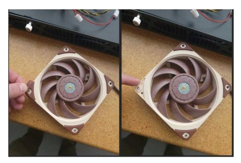
b. [Images 3 and 4 demonstrate installation of vibration plate.]
