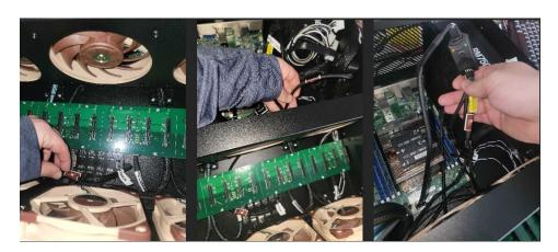
10. take another extension cable and plug one end into the fan controller and one end into fan header fan 1, fan 2, fan 3, or fan 4. [DO NOT PLUG INTO FAN A, FAN B, or FAN C.]
