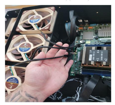
5. Ensure fan hub is plugged into fan controller, and the fan controller is plugged into a fan header fan 1, fan 2, fan 3, or fan 4 on the motherboard as shown in the front panel assembly [DO NOT PLUG INTO FAN HEADERS FAN A, FAN B or FAN C].
