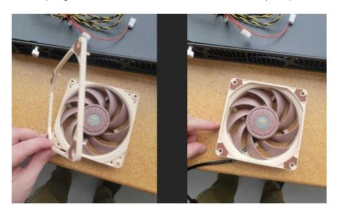
3. Starting with the HL-15 rear fan bracket, place "Fan Screws" into all 12 mounting holes and secure all with AP-1003W-B (rubber grommet) on the red side
