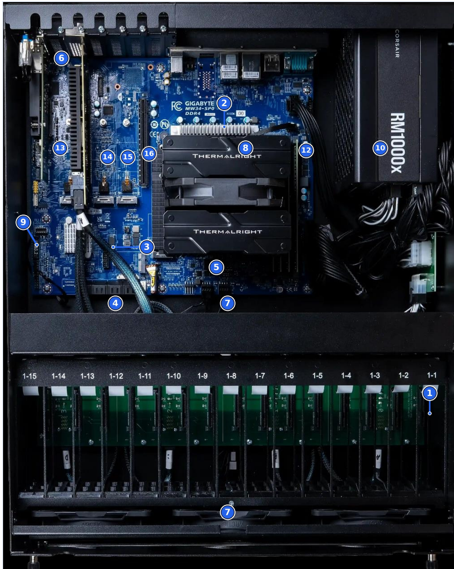
Figure 1: Internal layout – motherboard, RAM, PSU, and 15-bay backplane.
