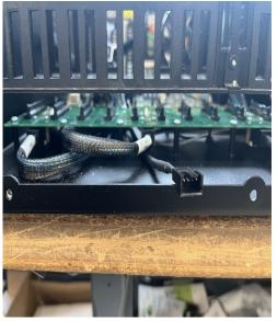
3. Take magnetic fan hub and connect the female end of extension cable to Fan Hub as shown.
