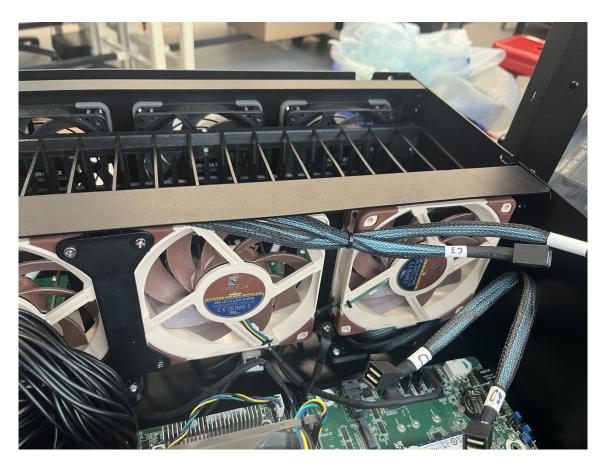
8. Route the other 2 cables into the **right most slot** of the center fan bracket assembly as shown.
