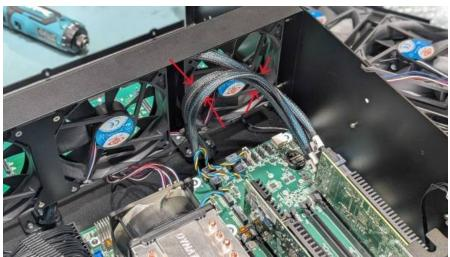
5. Carefully cut out the zip ties, fan wires are tied to.
