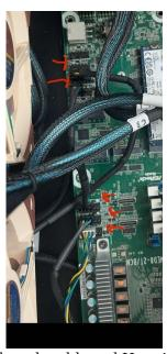
11. Connect the Motherboards cable and Heatsink's Fan if removed.
