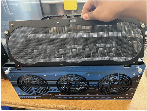
12. Remove the 7 screws from the front plate.
