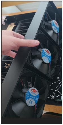
8. Remove the 12 screws securing the fans to the bracket.
