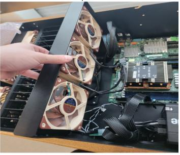
4. Once center bracket is placed into the chassis, use the 2 screws that were used previously to hold the center bracket and screw them into the chassis/center bracket to secure it into place.
