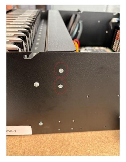
7. Slide the center bracket upwards and remove it from the chassis.
