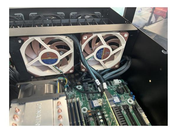
10. Connect all the fan cables to the motherboard's fan headers.
