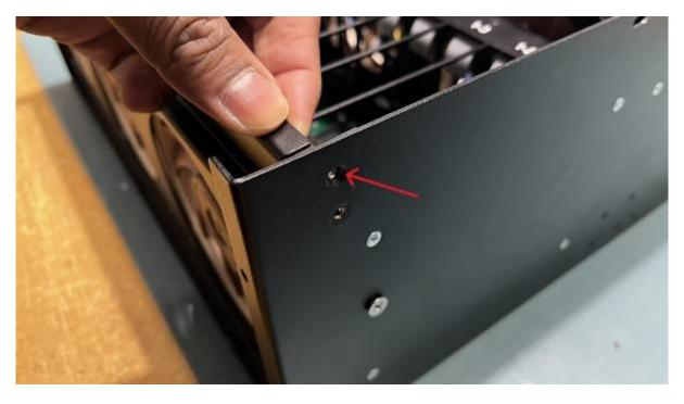
10. Insert screws in the mounting holes on the left and right side of the Chassis from the outside to fasten the Front Fan Bracket to the Chassis.
