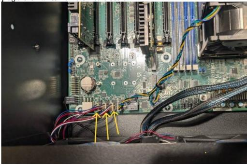
2. Disconnect the motherboard cables and remove heatsink fan, this will make it easier to remove the 3D-printed part or skip to step 3.
