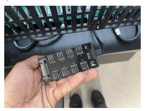
4. Place the Noctua Fan hub on the front end of the chassis back of PCB backplane as shown
