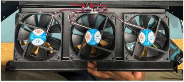
17. Unscrew the fans from the front fan bracket.
