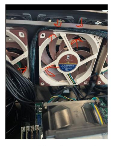
7. Align the 3D-Printed" part on to the holes of "Center Fan Bracket Assembly and screw it using fan screws
