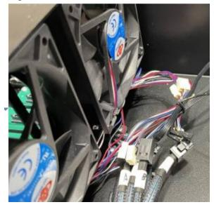
6. Unscrew the center fan bracket from either side of the Homelab chassis.
