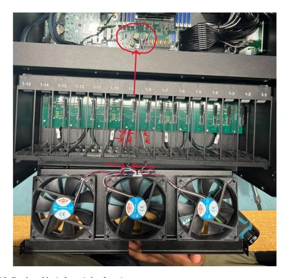
16. Cut the cable tie from tied to fan wires.
