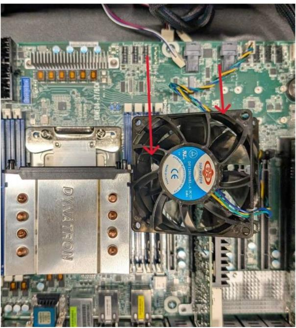
6. Route the SATA cables **A & B** through the channel in-between the fans from the other side as shown
