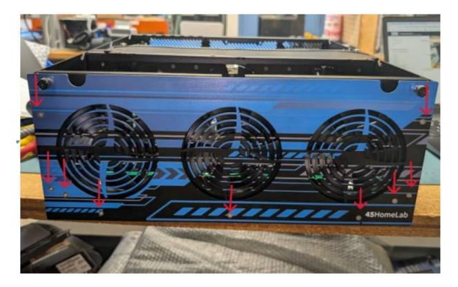
13. Unscrew the front fan bracket from either side of the Homelab chassis.
