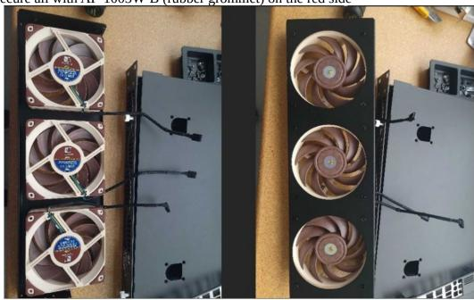
3. Slide the center bracket downwards and place it in the chassis.
